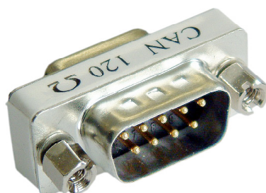
Picture 4-2: CAN bus termination resistor
