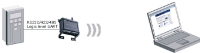
Figure 1. The gateway connected to the controller communicates wirelessly with a Bluetooth enabled Laptop.
